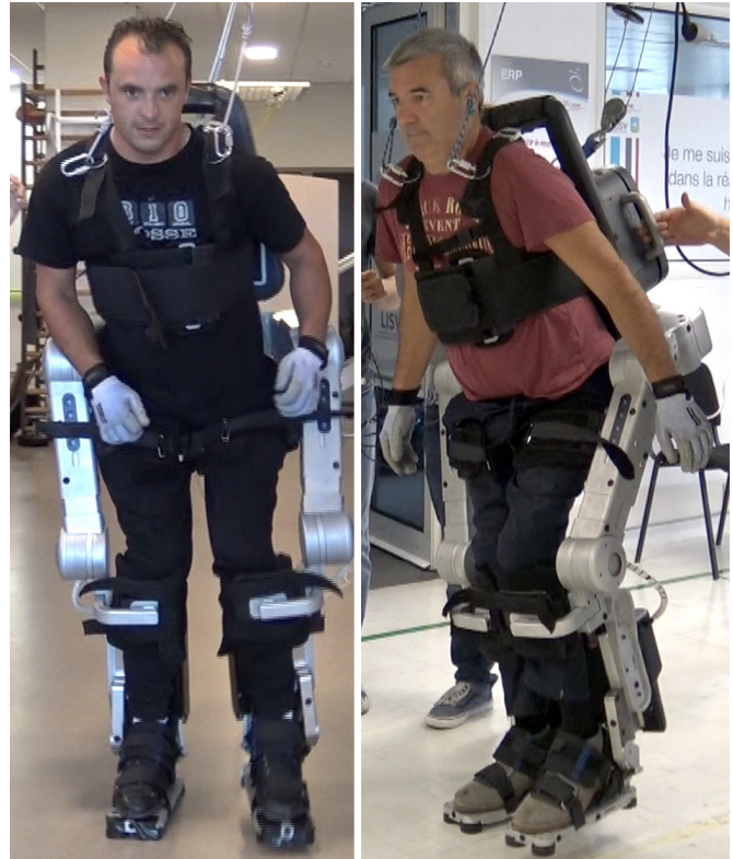
Fig. 1: Image of two paraplegic patients walking in the ATALANTE exoskeleton developed by Wandercraft.
