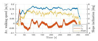
Fig. 8. Digit walking upslope in outdoors environment. The velocity profile demonstrate the robot keeps walking forward  $(v_x)$  while moving consistently upslope with almost no drift in the lateral direction  $(v_y)$ . The walking gait is robust to the varying inclination of the terrain, which is estimated by the FK-based slope estimator.
