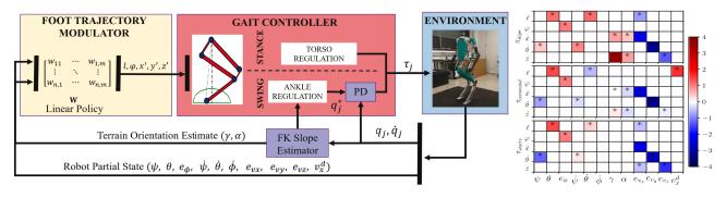
Fig. 3. Figure showing the control framework (left) and the policies (right) trained for walking 1) on arbitrary slopes, 2) on velocity command control, and 3) on stairs. In the policy matrices, the symbol '\*' marks the terms that were allowed to be non-zero, to be optimised through ARS. The final values of the learnt policy is shown as the colour map.
