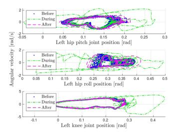
Fig. 10. The phase portraits of the joints are perturbed during the disturbance, but converge to the nominal walking limit cycles by the actions of the learned policy.
