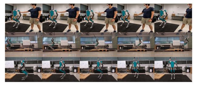
Fig. 6. Tile plots of Digit recovering from a external push (top), blind walking on terraced surface (centre), and turning in place as per command (bottom) using the learned linear policies.
