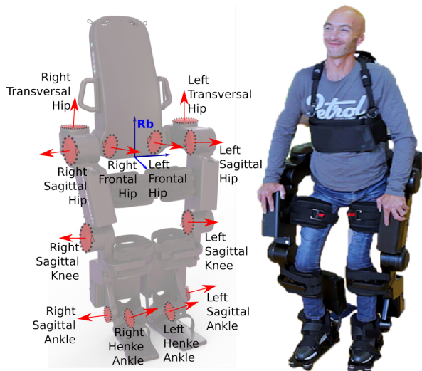
Fig. 1: The ATALANTE exoskeleton and its kinematic tree structure, where R_b is the floating-base coordinate located at the center of the pelvis.
