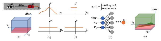
Fig. 1. Example for some of the definitions introduced in Section II. (a) Standard lead-vehicle following testing system and its corresponding OSS design. (b) Example of Type-I difference. (c) Example of Type-II difference w.r.t.  $\mathcal{TE}^u$ . (d) Example of Type-II difference w.r.t.  $\mathcal{TE}^{\pi}$ . (e) Conceptual illustration of the almost safe set.
